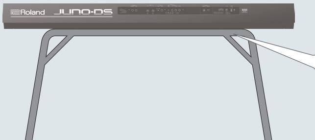
Adjust the width of the stand so that the rubber feet of the JUNO-DS fit into the rubber foot receptacles
