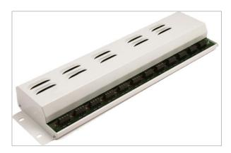
Support engineers should install the relevant driver for the Measurement Computing unit. The driver should be installed by default on a dCine, however the driver installer can also be downloaded from the digitAll website. Once the driver is installed and the device has been connected, support engineers will need to detect the device using a utility that comes with the driver installer called InstaCal.
