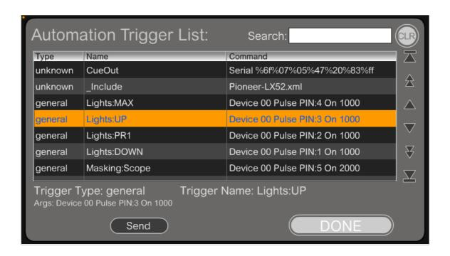
You can use the List All button to search for a defined Trigger. After pressing List All you will see the "Trigger Type:" and the "Trigger Name:". This tells you how the trigger will appear on the automation button screen. The "Args:" section describes exactly what the trigger will do. The above diagram includes an example for the "Args:" for Lights:UP-
