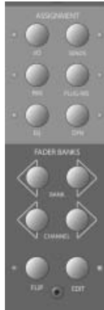
Figure 74-10: The Assignment section gives you access to plug-ins, I/O assignments, sends, and other track parameters.
