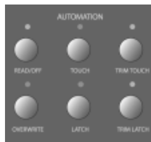
Figure 74-13: Change a track's automation mode with these buttons.
