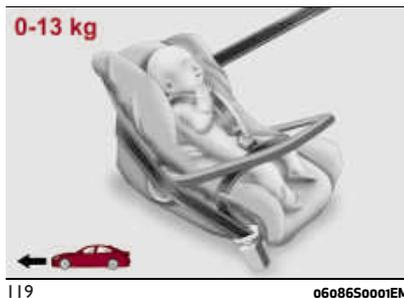
The child restraint system is restrained by the car seat belts, as shown in fig. 119 and it must restrain the child in turn with its own belts.
