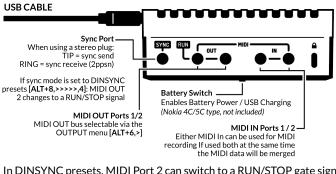
In DINSYNC presets, MIDI Port 2 can switch to a RUN/STOP gate signal for extra synchronization. You can e.g. use our RK-TRSPLIT cable to use both signals.
