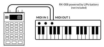
Above you can see a simple setup to add MIDI recording to a Synth. If you connect the RK-008 on a single MIDI device: Make sure 'MIDI Local control' on your device is set to 'off' to prevent note doubling. If this is not possible you can disable the direct MIDI output of the RK-008 by disabling the ROUTE option to prevent MIDI loops.
