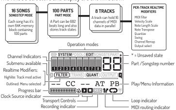
If you want the RK008 to slave to a gate signal, set the clock source to AUTO (ALT+8,>,>,5) and the metronome icon will light up. The RK-008 uses upscaling to generate a MIDI clock from these lower rate pulses.
