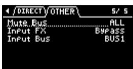
**4. Use the [VALUE] knob to move the cursor to “Input FX”, and press the [VALUE] knob.**
