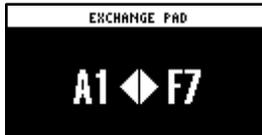
2. **Press the two pads for which you want to exchange the samples.**
