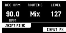
4. **Turn the [CTRL 3] knob to adjust the volume of the audio input.**
