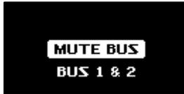
3. **To turn MUTE BUS off, hold down the [SHIFT] button and press the [BUS FX] button again.**
