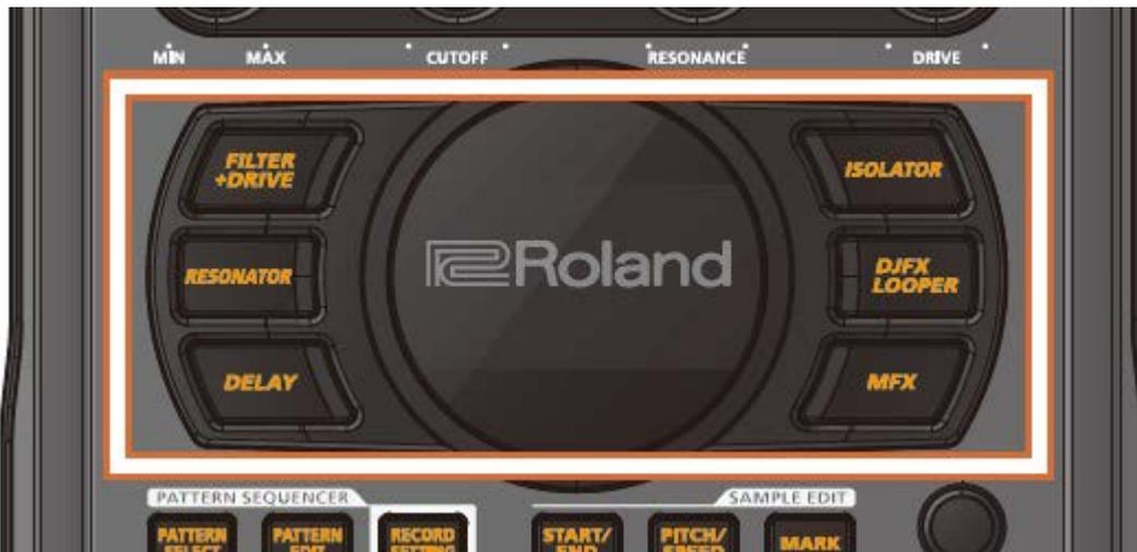
Press the buttons of the effects you want to apply, including the [FILTER+DRIVE] button, the [RESONATOR] button, the [DELAY] button, the [ISOLATOR] button, the [DJFX LOOPER] button, and the [MFX] button. This turns the effects on.
