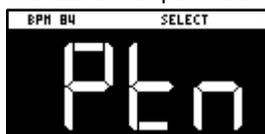
3. While holding down the [HOLD] button, press pads [1]–[16] to select the pattern chain number (1–16) to record.
