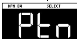
2. While holding down the [HOLD] button, press pads [1]–[16] to select the pattern chain number to play back.
