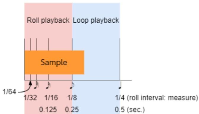
When the roll interval is set to 1/64–1/8, the sample plays back as a roll.
