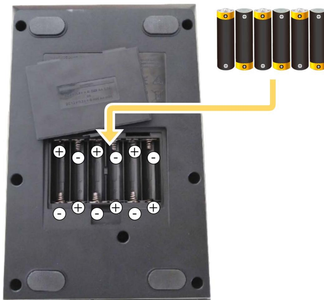
This unit uses six AA batteries (rechargeable Ni-MH or alkaline).
