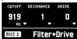
The display switches between main parameters and sub-parameters each time you press the [VALUE] knob, depending on the effect.
