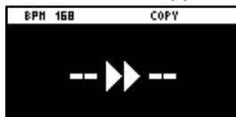
2. **Press the pads in order, beginning with the pattern (pad) you want to copy, and then the copy destination pattern (pad).**
