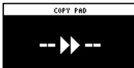
2. **Press the pads in order, beginning with the pad you want to copy (sample), and then the copy destination pad.**
