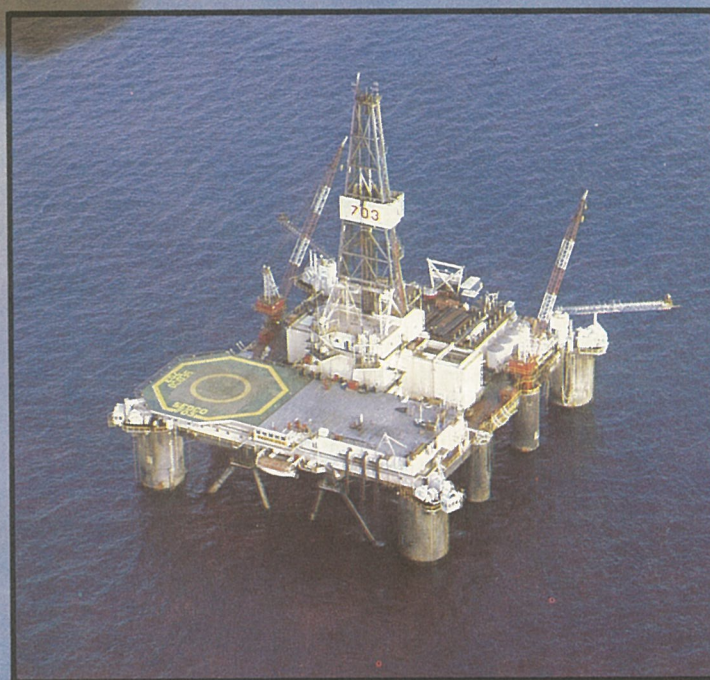
Above: An oil production platform (rig) in the North Sea. These platforms have to be able to withstand winds of up to 200 kilometres per hour and waves up to 30 metres high.
