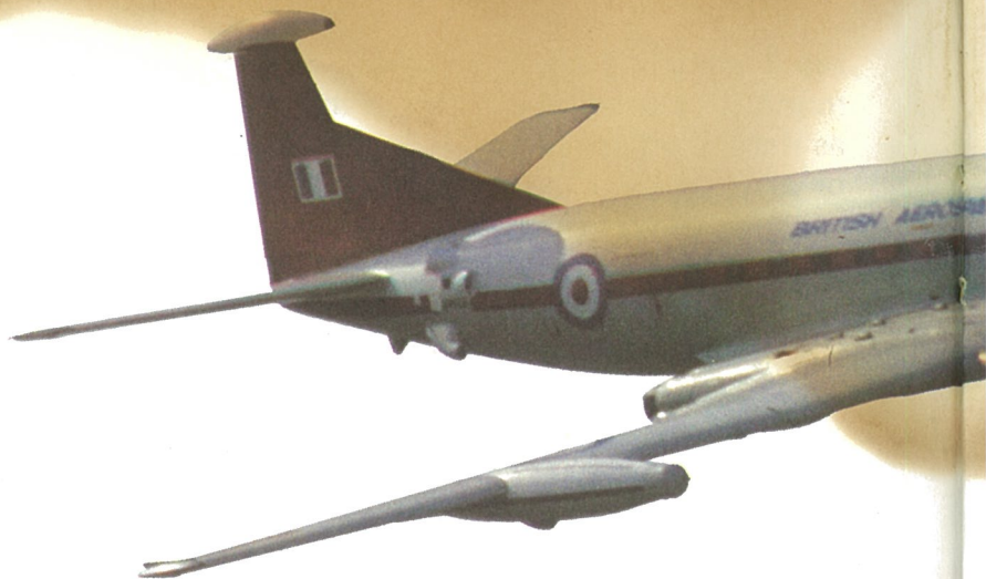
Above: The strange radar nose on this aeroplane allows it to keep track of other aeroplanes over a very wide area.
