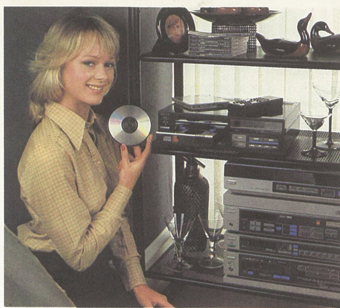
Above: Compact discs are read by a laser beam rather than by a needle. This means the disc is not actually touched by anything except a light beam and so is very long lasting.
