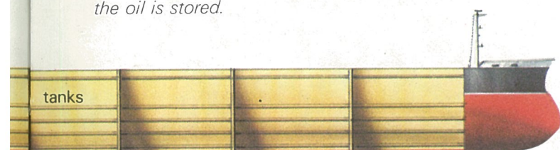
An oil tanker cut-away to show the huge tanks where the oil is stored.
