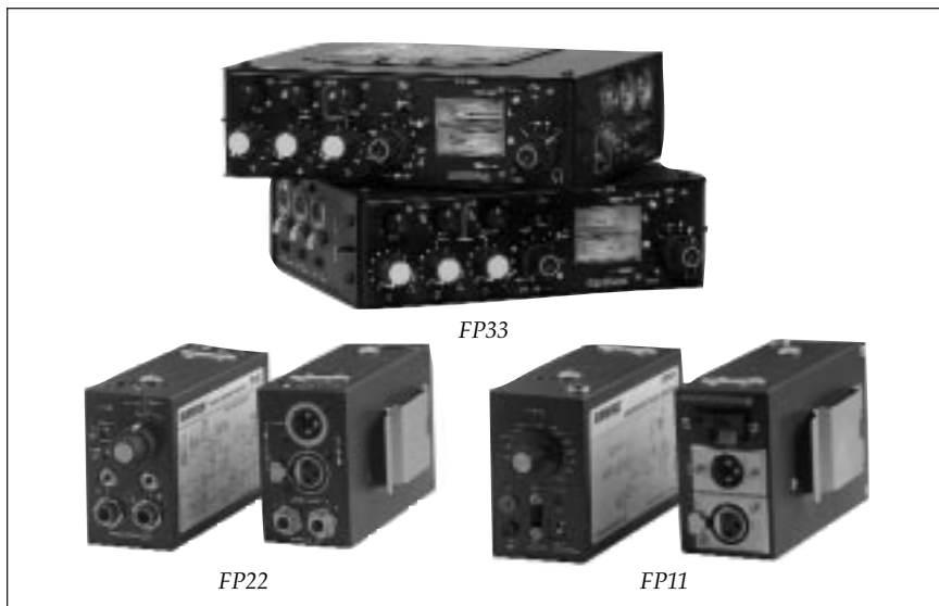
Examples of a portable stereo mixer (Shure FP33 shown above), headphone monitor (Shure FP22 shown bottom left) and mic-to-line amplifier (Shure FP11 shown).
