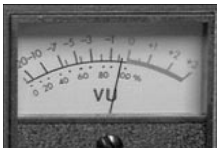
Average reading if level is properly set.
